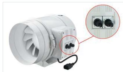
The fan with the electronic module of the temperature sensor and the speed controller is used for automatic speed control (air capacity regulation) depending on the air temperature in the ventilation duct or inside a room.
