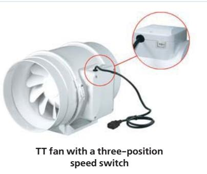
The double-speed motors are controlled with a built-in switch (V option) or an external switch for multi-speed fans (available upon separate order). An integrated speed controller (option P), an external TRIAC or autotransformer speed controller (available upon separate order) are used for smooth speed control when connected to the maximum speed terminal.
