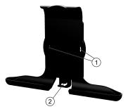
Fig. 2 Holder for NaviPad, (1) fixing points, (2) cable hook
