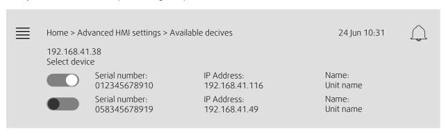
The air handling unit will appear, press the button to select the air handling unit to pair it with the NaviPad. If there are several air handling units at the same IP subnet, a list of available air handling units will be presented.
